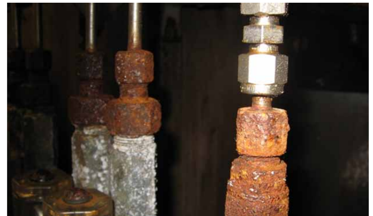
Galvanic reaction created by mixing different body & nut materials.
