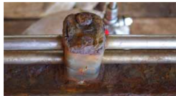
Crevice corrosion between the tube/tube trap interface.
